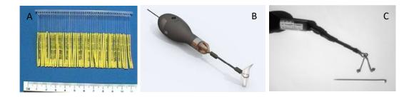
Figure 2. A. T-bar Tags; B. Electronic satellite tag (PAT); C. Anchor designed and used in this study.
